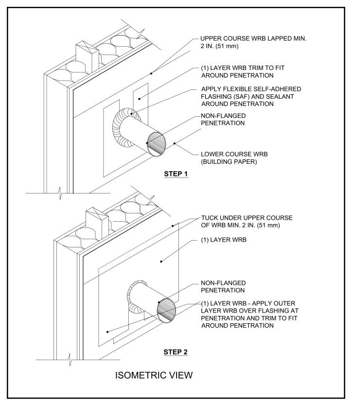
Flexible self-adhered flashing and WRB installed in a watershed fashion help prevent water infiltration.
