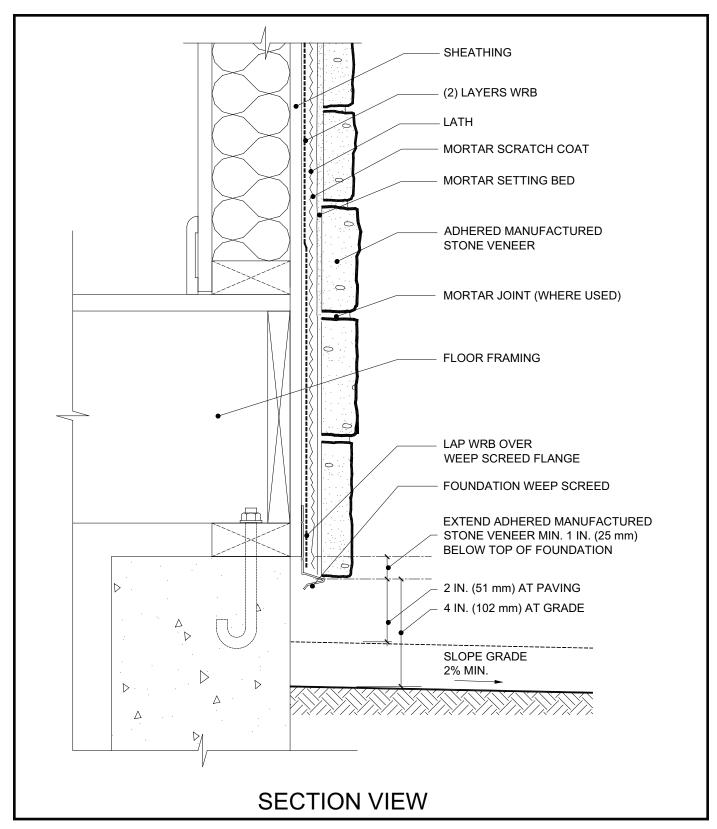
A minimum 4 in. (102 mm) gap is required at the base of the stud wall to grade and a minimum 2 in. (51 mm) gap is required at base of the stud wall to a paved surface.
