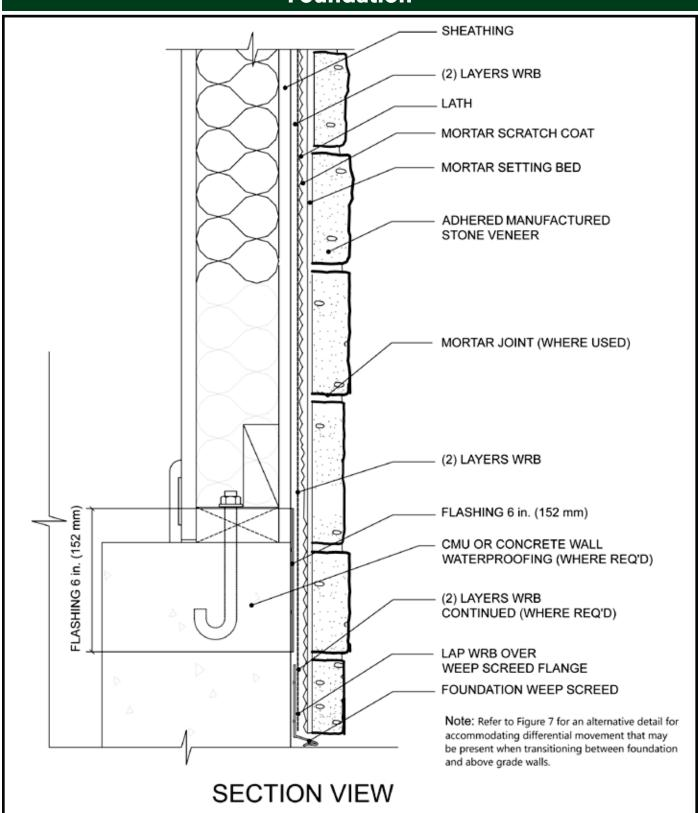
AMSV may overlap foundation wall with careful installation of flashing and WRB. This installation may continue down foundation wall to grade clearance.
