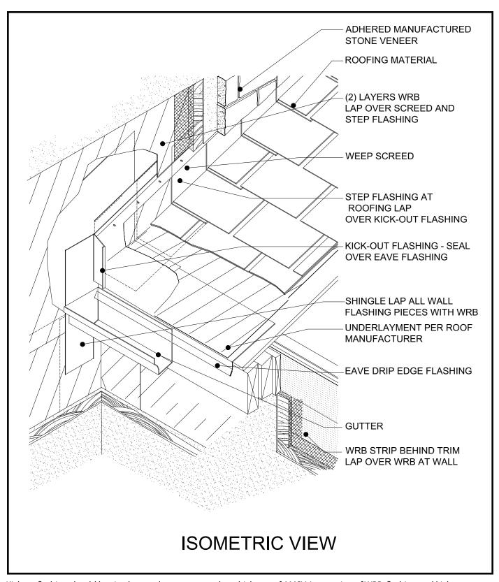
Kickout flashing should be sized properly to accommodate thickness of AMSV. Integration of WRB, flashing and kick-out critical.
