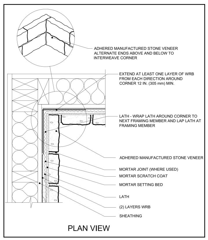
Randomly alternate ends above and below to interweave the corner. Double wrap water resistive barrier around both sides of the corner. Lap lath to the framing at least 12 inches (305 mm) to the next framing member.
