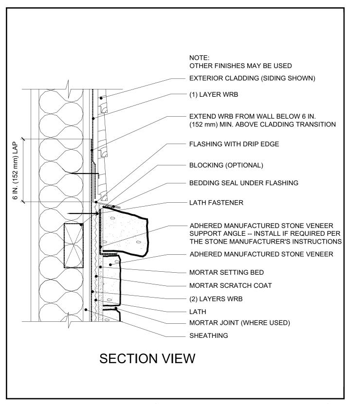
Flashing should be installed prior to the adhered manufactured stone. Water resistive barrier laps over the vertical leg of flashing for positive drainage. Optional support angle shown. Verify installation requirements with adhered manufactured stone veneer manufacturer.
