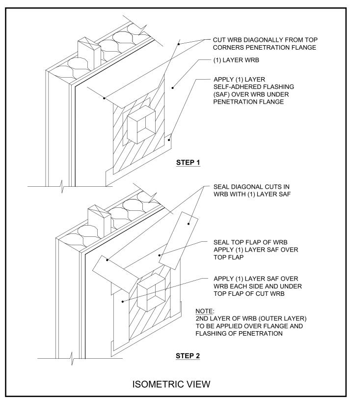
Penetration with flanges can be incorporated into the wall system by applying WRB in a watershed fashion and sealing cuts in the WRB with self-adhered flashing. Drawing illustrates installation with housewrap WRB. Installation with building paper WRB would be similar but instead of 45 degree cuts, fit last piece of WRB on top of flanges and tuck under WRB course above penetration (similar to Step 2 in Fig. 31.).
