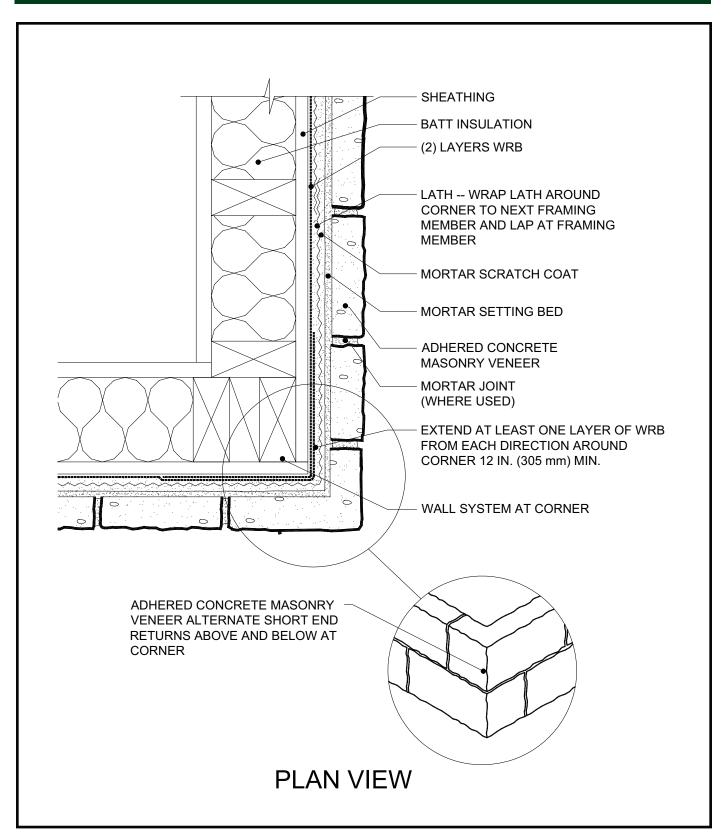
Randomly alternate short end returns above and below at the corner. Lap lath around the corner to the next framing member.
