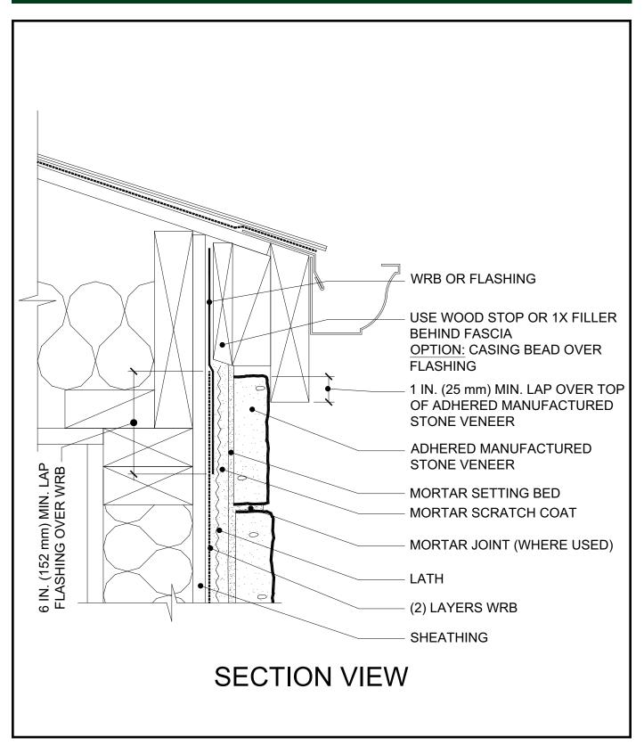
Water resistive barrier should be in place prior to soffit installation followed by adhered manufactured stone veneer.
