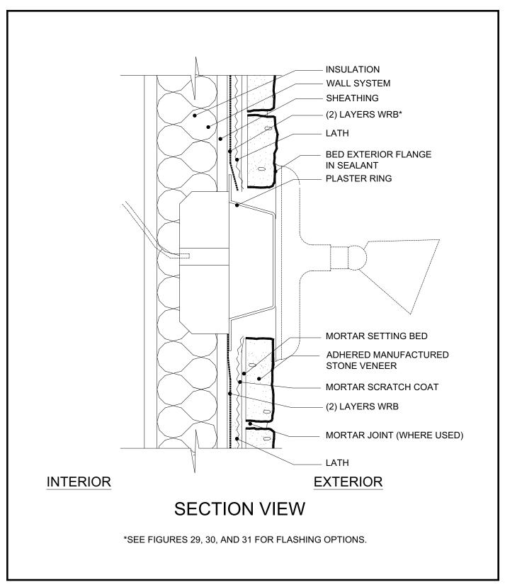
Plaster rings should be affixed over the service box to bring the face of the box flush with the adhered manufactured stone veneer. Bed the exterior flange in sealant. Water resistive barrier should be installed snugly around the plaster ring flange.
