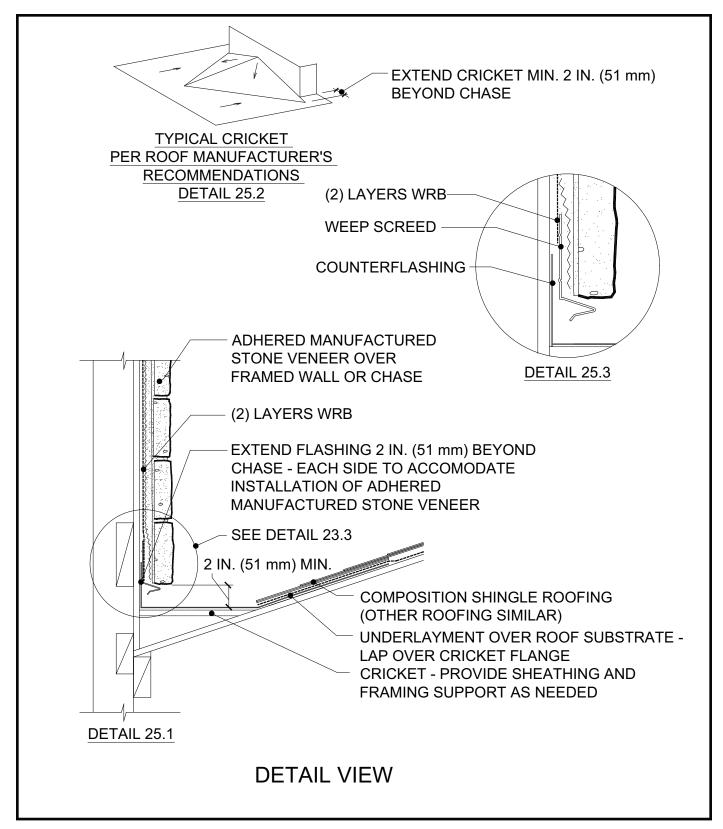
A cricket up-slope of a roof penetration, such as a chimney, helps direct water around the penetration.
