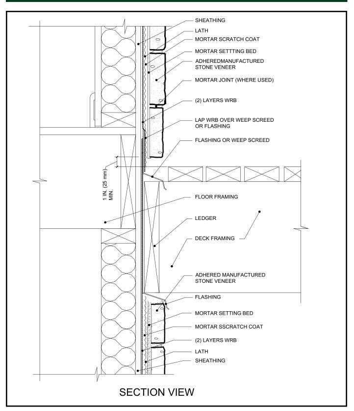
Lap water resistive barrier over weep screed and floor framing to manage water intrusion. Provide gap between adhered manufactured stone veneer and decking for drainage. Water management at the deck ledger boards is critical, and may vary based on the building design.
