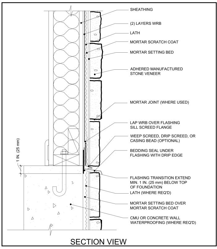
AMSV may continue down the foundation with the incorporation of a flashing transition with careful installation of WRB and flashing.
