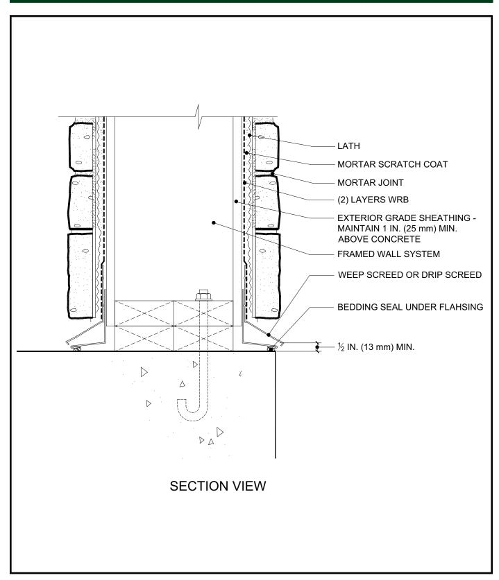
A minimum one half inch (13 mm) clearance should be maintained at all sides of the base. All column materials to be exterior grade. Do not extend flashing past edge of AMSV for safety reasons.
