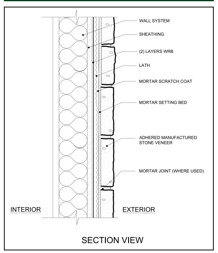
Note: layering of sheathing, water resistive barrier, lath, scratch coat, and adhered manufactured stone veneer.
