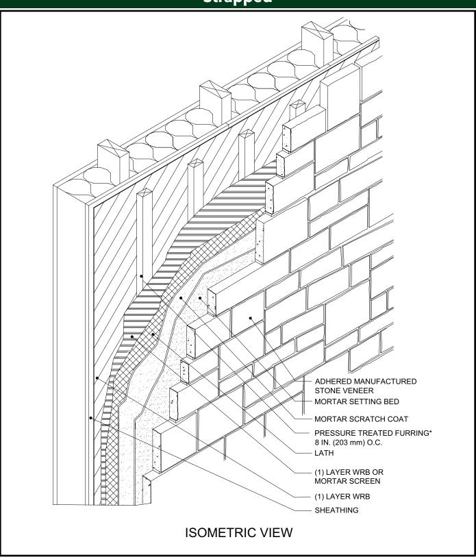
A rainscreen system of vertical strapping / furring creates a vertical gap between the primary WRB and the mortar screen / WRB on the back of the scratch coat. \*Furring fastened into framing and into nailable sheathing between framing.
