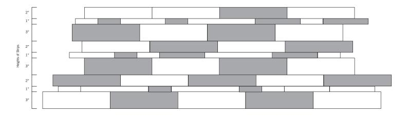
The vertical layout of strips in each row shows this pattern: 3", 1", 2", 3", 1", 2".. etc. It is best to keep all vertical rows with the same height of stones.
