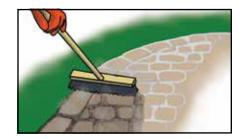
4. **Blow off** any remaining Polymeric Sand on paver pores and crevices.
